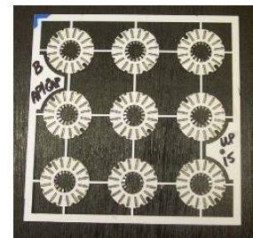
(c) 128 x 128 mm panel of GGA arrays Without fuel and final backing layer
