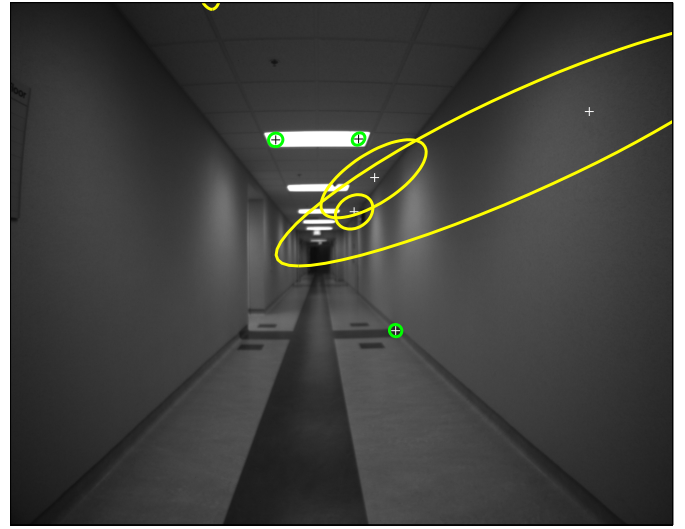
Figure 6: Sample image from indoor data collection. The indoor data collection presented the filter with man-made features in an office environment. The crosses and ellipses indicate the locations and uncertainty of currently tracked landmarks.
