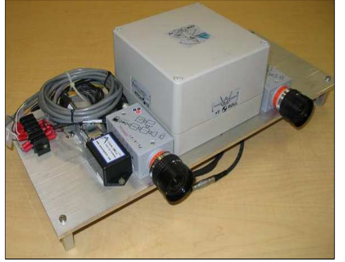
Figure 4: Data collection system. The data collection system consisted of a tactical-grade IMU and monochrome digital cameras.
