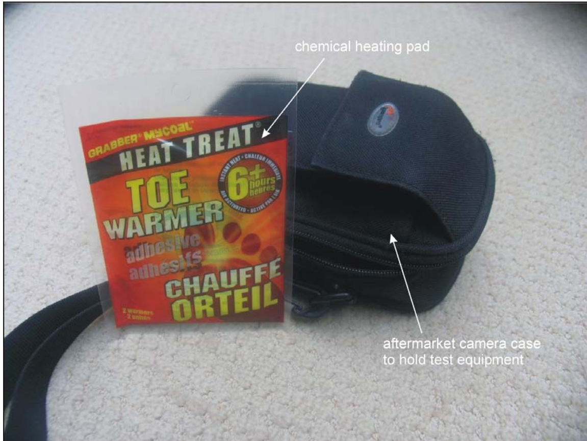
Figure 2: Chemical heating pad with aftermarket camera case.
