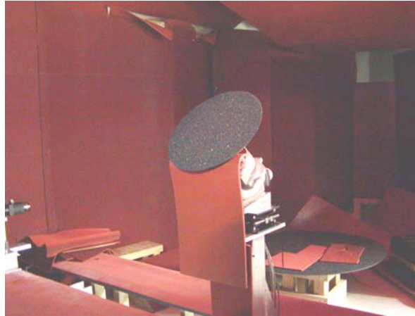
Figure 4. Ground plane CN mounted in the W-band compact range.
