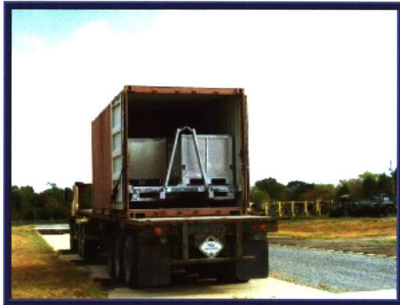
Photo 1. Hazard Course Testing of the JMIP in the Intermodal Container.
