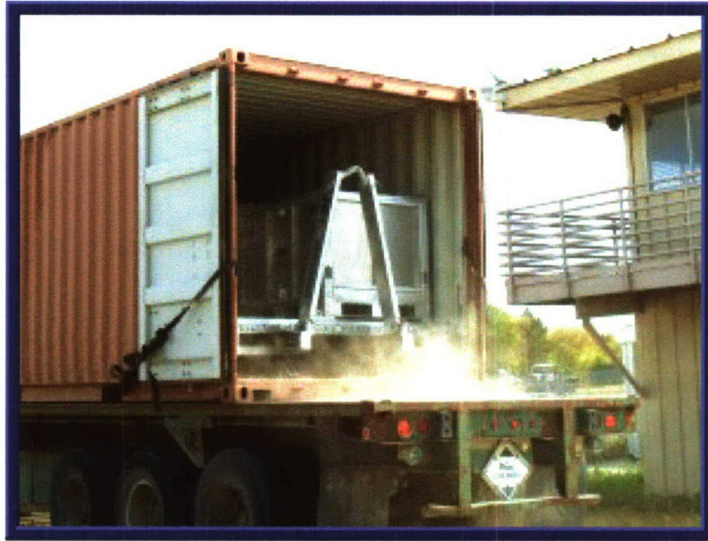
Photo 3. Washboard Course Testing JMIP.
