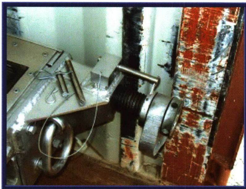
Photo 8. Sheared Pin and Disengaged Cam
