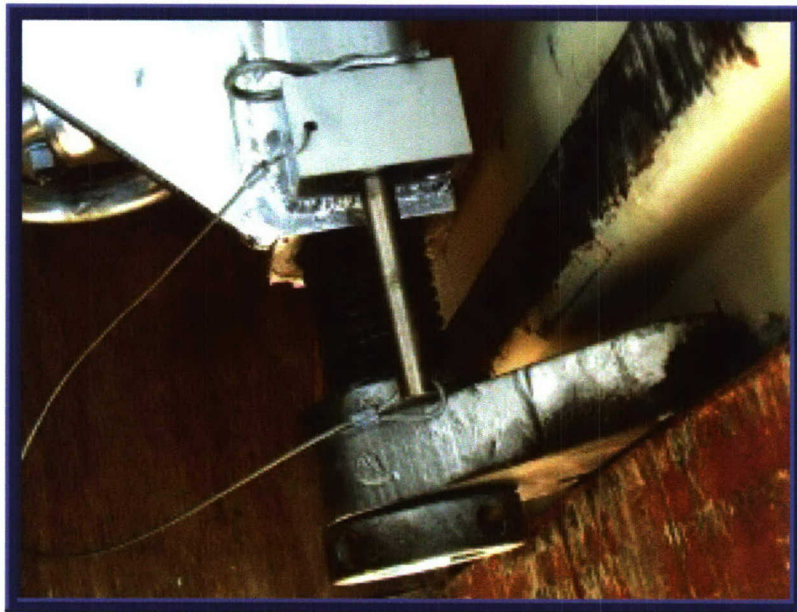
Photo 5. Pin not Properly Engaging Cam.
