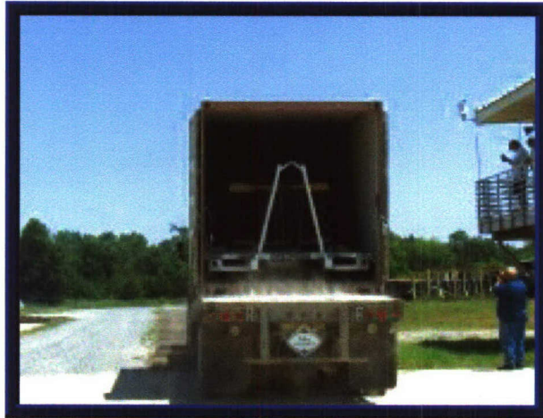
Photo 10. Washboard Course Testing of the JMIP.
