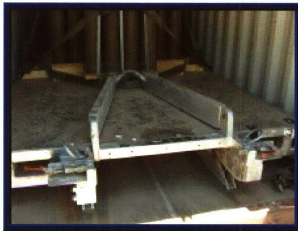
Photo 11. Collapsed A-frame from Failed Pin.
