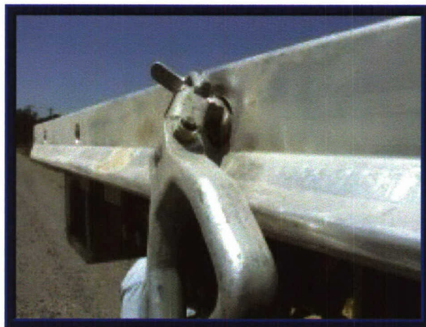
Photo 4. Loose Tie-down Ring.
