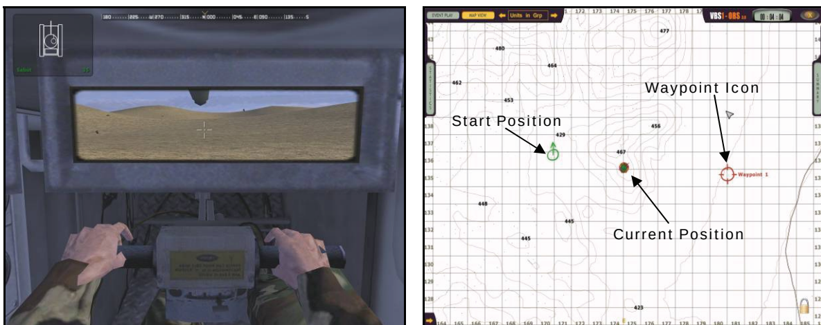
Figure 9. Moving map displays: primary display showing GPS and compass (left) and waypoint display (right).
