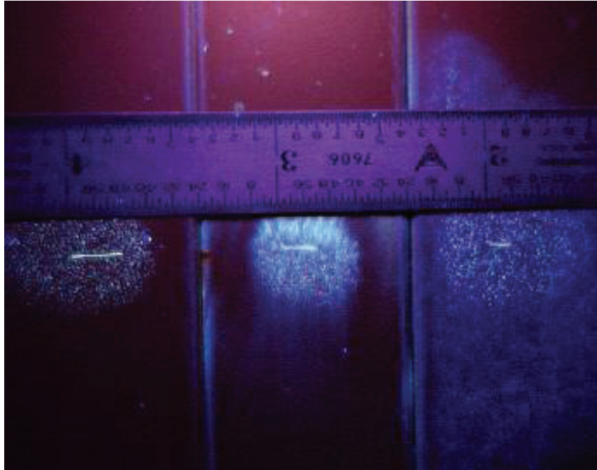
Figure 24. FPI micrograph of cracked Mg bar nos. 3, 6, and 7 after crack extension under the coating system. Cracks can be observed; however, the absorption of the penetrant by the coating is still evident.
