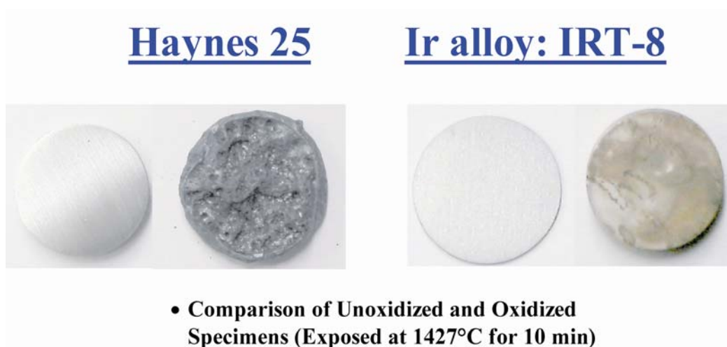
Figure 14. Results of Oxidation Test of Iridium Alloy
