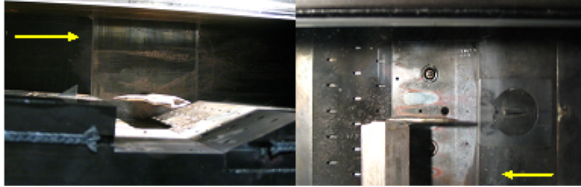
Figure 4. Cone-static probe installed in the tunnel
