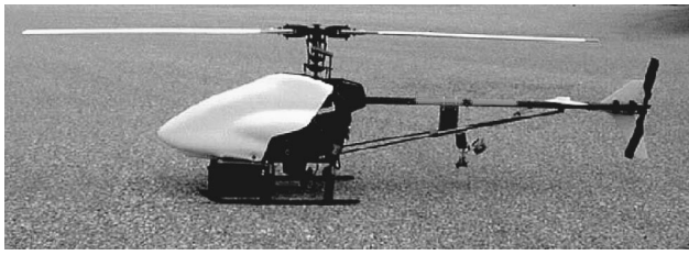
Fig. 9 The small UAV used in the NRL field tests is shown. The payload was attached to the tail and was designed to be lightweight but flexible to accommodate different experiments.
