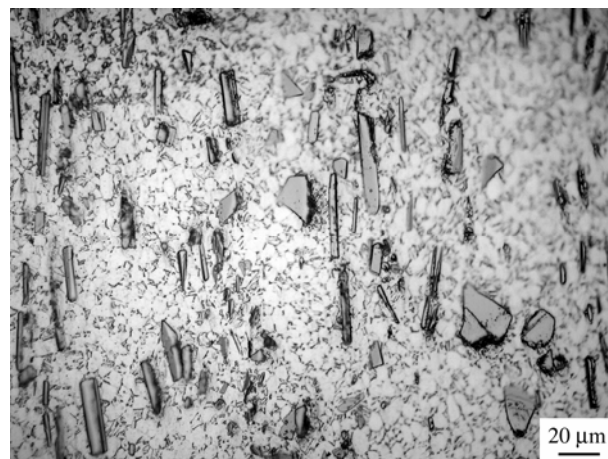
Fig. 4 Microstructure of Ti64-1.55B in “1D” beta-forged / \alpha+\beta rolled condition.
