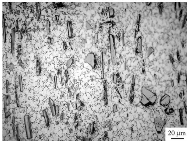
Fig. 6. Globular matrix in "1D" beta-forged / \alpha+\beta rolled Ti64-1.55B material.
