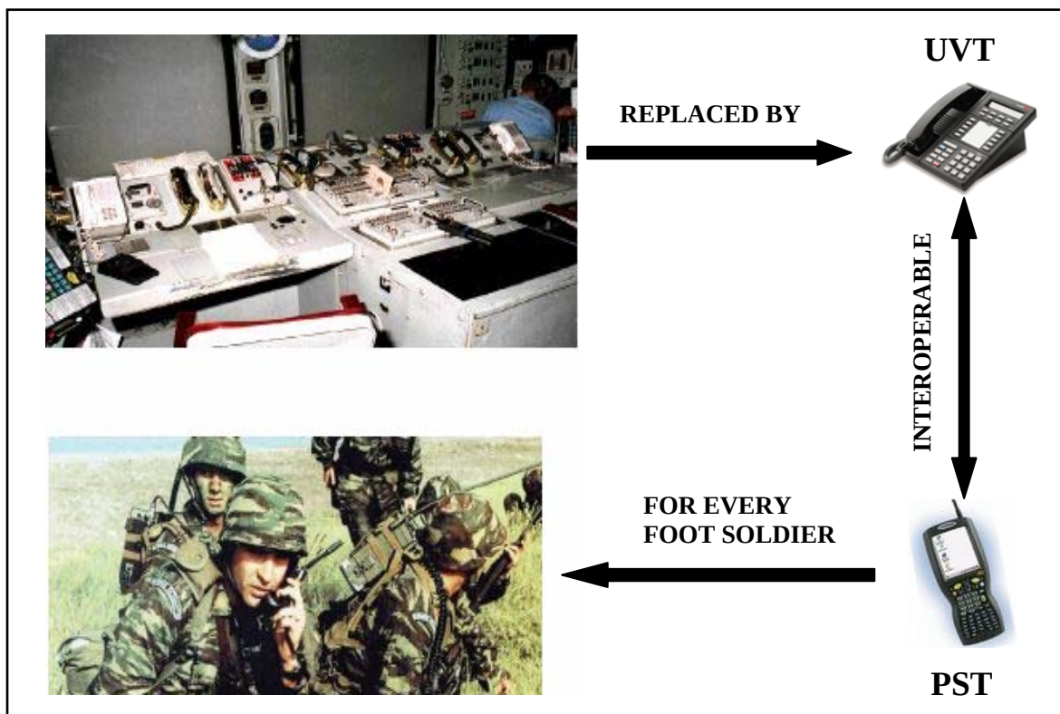
Fig. 1 — Combat Information Center (CIC) with a confusing array of secure voice terminals. VDR can integrate all these incompatible voice terminals into a single interoperable secure voice phone that we call the Universal Voice Terminal (UVT). In addition, we plan to develop a pocket-size version of VDR for every foot soldier that we call the Personal Secure Terminal (PST). PST gives connectivity among all soldiers and also interoperates with a UVT to reach the command center or other plant version of the VDR. Note that currently all soldiers are given weapons, but not a phone. In the future, every foot soldier should have a pocket-size phone that enables them to communicate with fellow soldiers and the commander. There should be no incident similar to that of Jessica Lynch who fell into enemy hands because of the inability to make contact with friendly forces.
