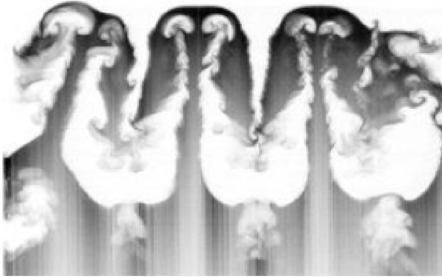
Figure 2.3: Rayleigh Taylor Instability image from http://web.arizona.edu/fluid-lab/rayleigh.html . A dense fluid is held aloft by a less dense fluid below. A perturbation can trigger overturning, leading to the production of lower density structures (bubbles) that rise through the denser fluid. In this figure, the dense fluid is white.
