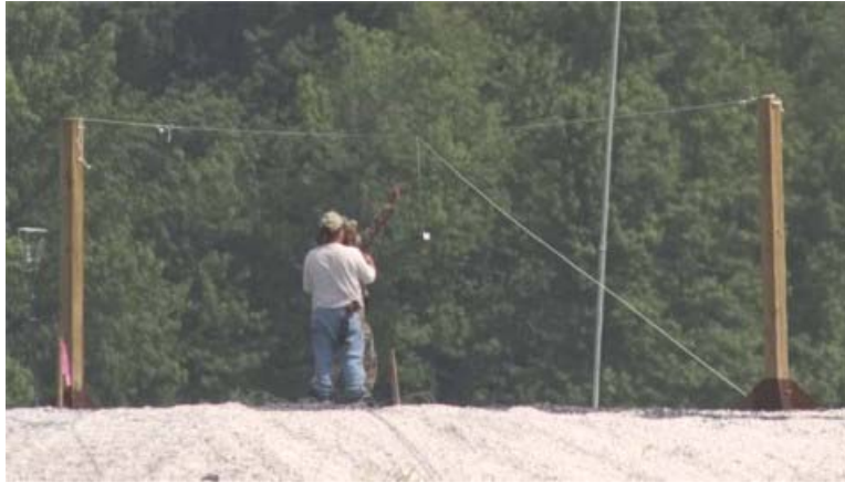
Figure 6. C-4 brick being suspended at 1.5 m above the gravel pad.
