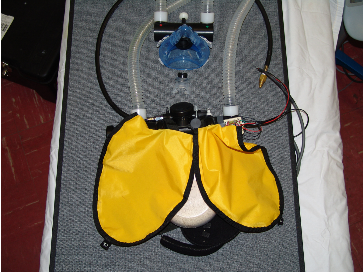
Figure 2: Photo of the modified MBS 2000 closed circuit oxygen rebreather. (See Figures 3 and 4 for more detail).
