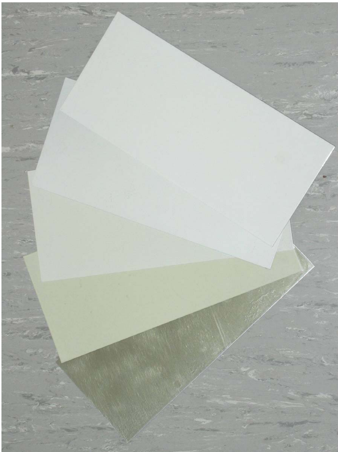
Figure 21; photograph of the UVB irradiated panels showing increasing discoloration with \text{TiO}_2 loading reduction.
