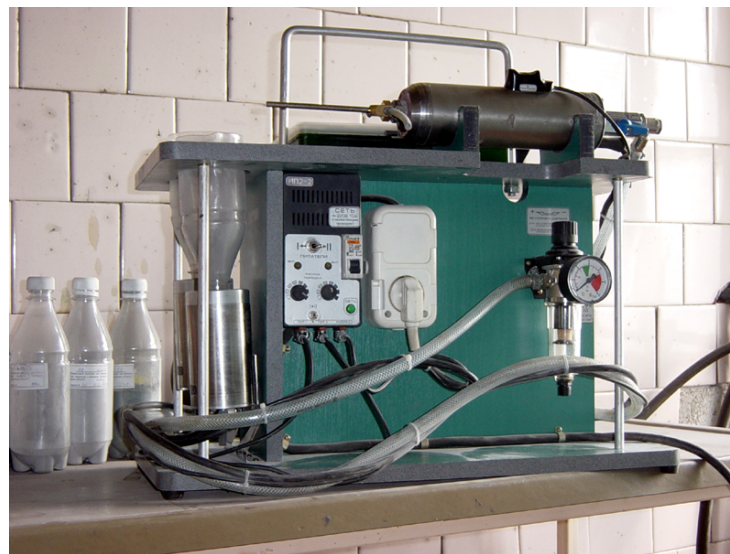
Fig .9 Schematic diagram and appearance of the installation for “cold” gas-dynamic spraying
