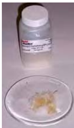
Figure 3: A) Trisilanolphenyl-POSS, B) first sample of Epoxy Cyclohexyl POSS (neat), C) second sample of Epoxy Cyclohexyl POSS dissolved in tetrahydrofuran (THF) at 50wt%.
