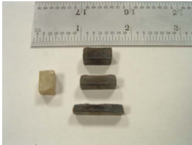
Figure 4.8: Channel Die Compression samples with original sample. This picture shows the finished products from the three 500°C runs set next to an undeformed sample. The three deformed samples are arranged from top to bottom in increasing degree of strain
