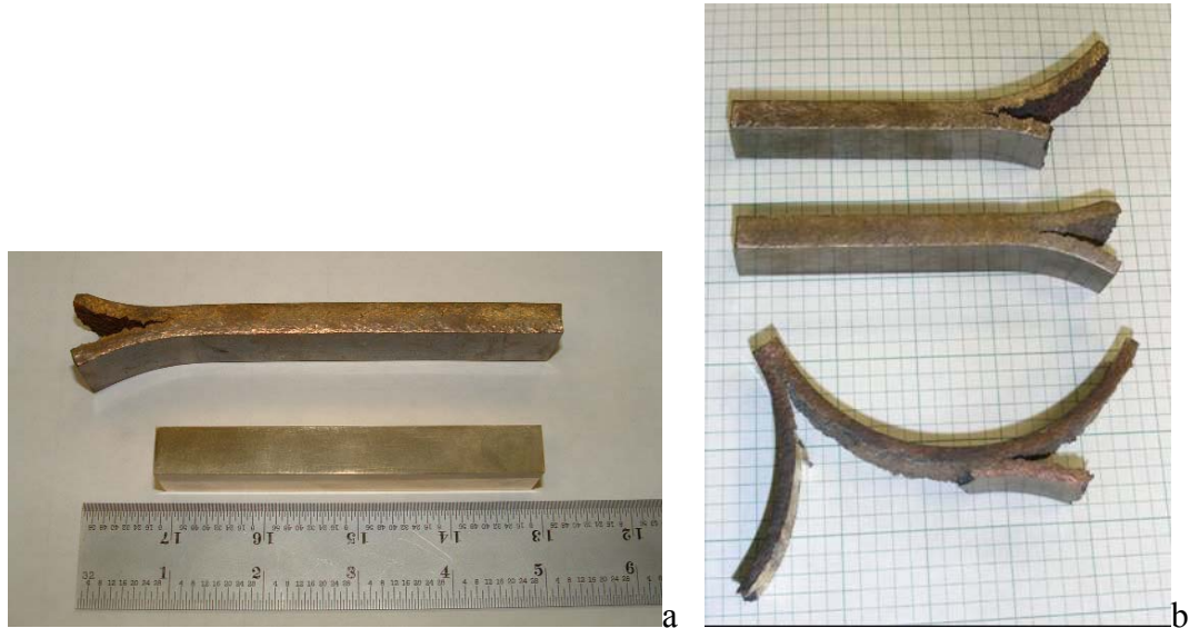
Figure 4.1(a & b): Rolling failures. Left – a 600°C rolling sample shown with an unaltered sample. Right – More examples depicting the difficulties of rolling NAB (400, 500, 650°C).
