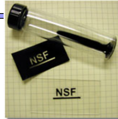
Ink (above), mask (middle) and printed image (bottom)
