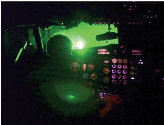
Figure 2: Cockpit glare induced by a 532 nm laser exposure ( 50 \mu\text{W}/\text{cm}^2 ).
