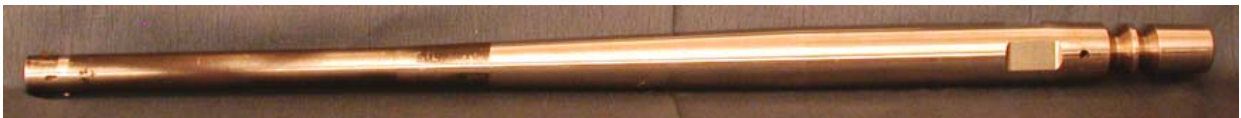
Figure 2. 20-inch sting extension used to mount wedge model near center of test section
