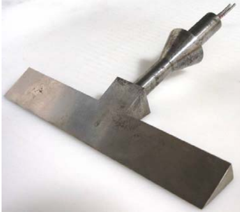
Figure 1. Flow angularity wedge used in shakedown and control calibration
