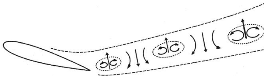
Figure 7.3.6 – Controlled airfoil wake pattern proposed by Wu et al. (1998).
