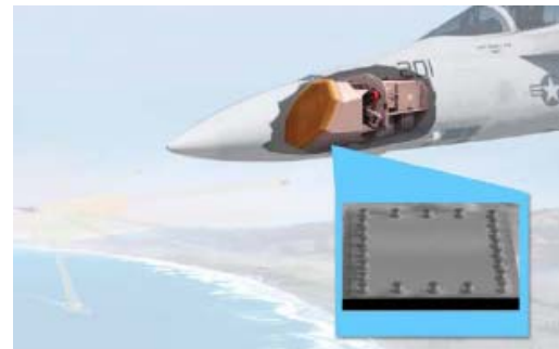
F/A-18 AESA Radar using die with Flip Chip bumps
