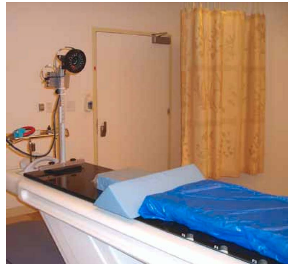
FIG. 3. The RPM infrared camera and illuminator system is mounted at the foot of the couch and used to track the motion of infrared reflectors placed on the top of the thorax phantom or the diaphragm of the patient.
