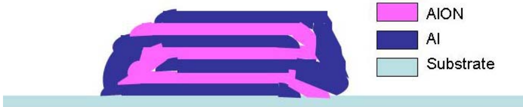
Figure 4. Cross-sectional schematic of AlON multilayer capacitor.
