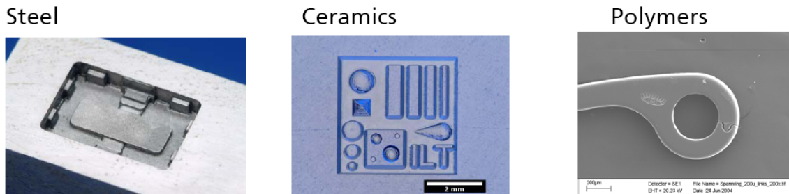
Figure D.34. Materials and shapes formed via laser ablation process.
