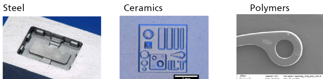
Figure 4.21. Materials and shapes formed via laser ablation process.
