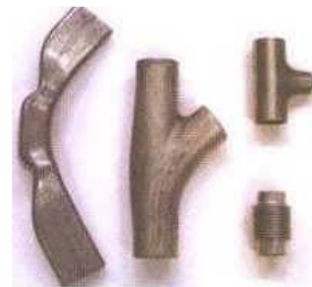
(c) Hydro-forming parts.
