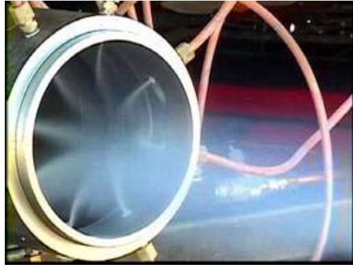
Figure 6. Liquid propane injection.
