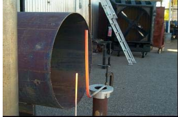
Figure 12. Controlled heat flux combustor operating at 1400°C.
