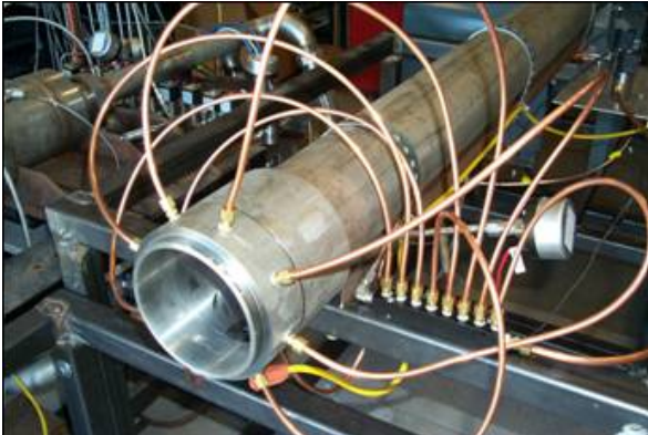
Figure 5. Liquid propane injection.
