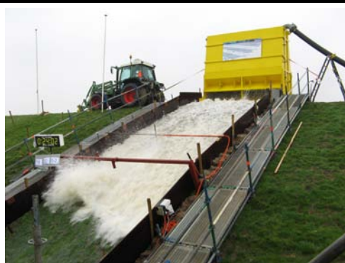
Figure 13 Recent field test in the Netherlands on the impact of overtopping waves on an existing levee.
