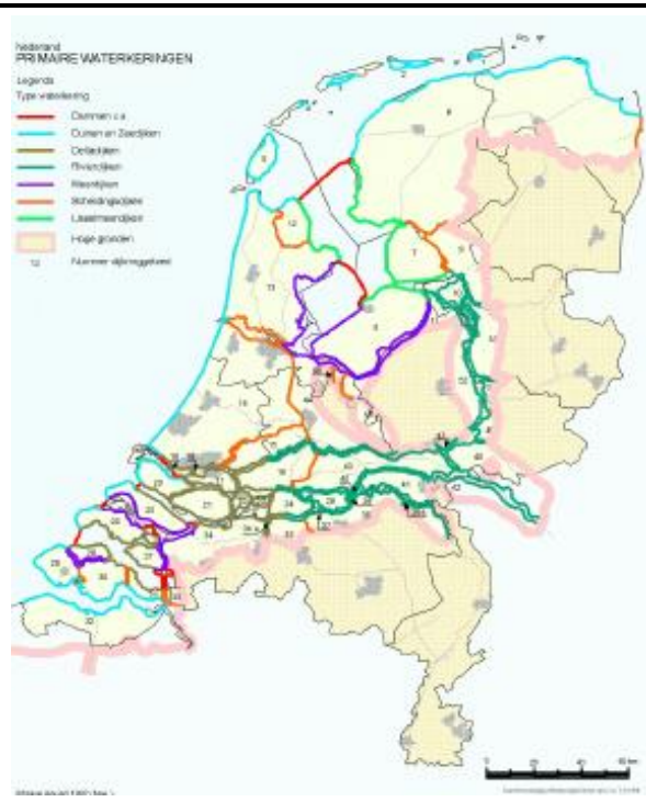
Figure 90 Primary flood protection structures
