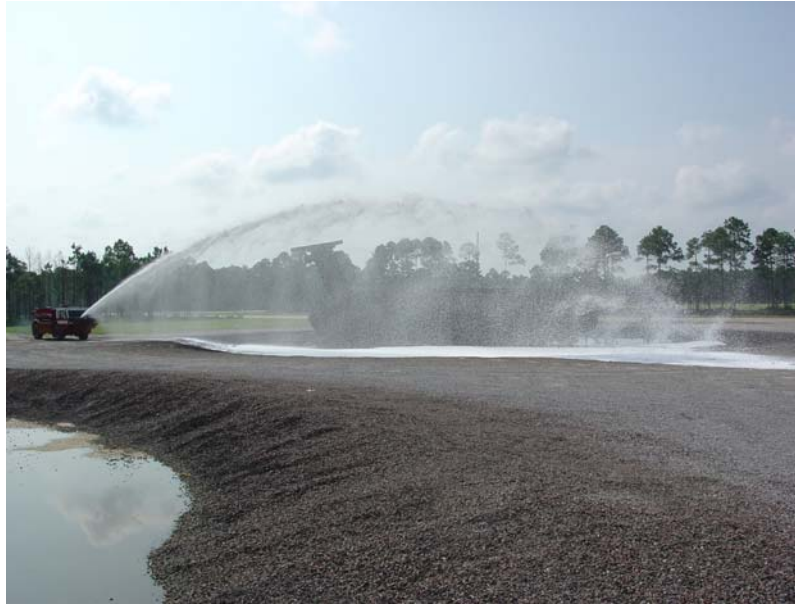
Figure 4.5.1: The Elkhart Brass UHP turret nozzle undergoing a throw test.
