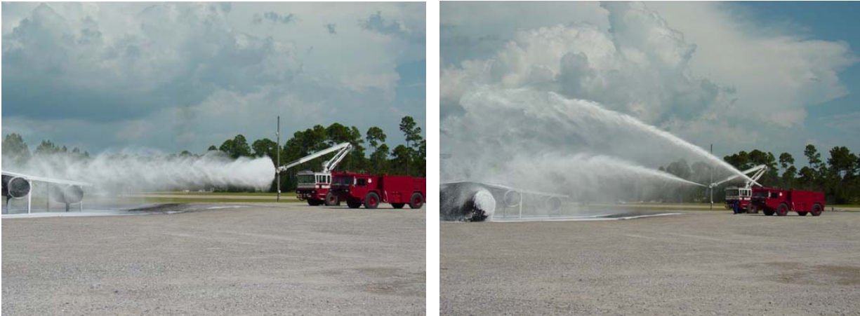
Figure 2.4.1: (a) The 200 gpm UHP Oshkosh T-1500 delivering agent. (b) Side by side comparison of agent streams (200 gpm UHP and standard 500 gpm P-19).
