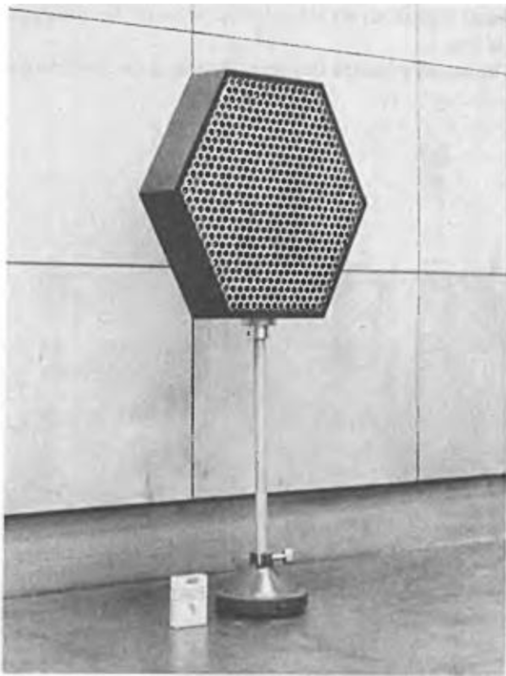
Figure 2. The first parametric loudspeaker from Yoneyama, et al. (1983).
