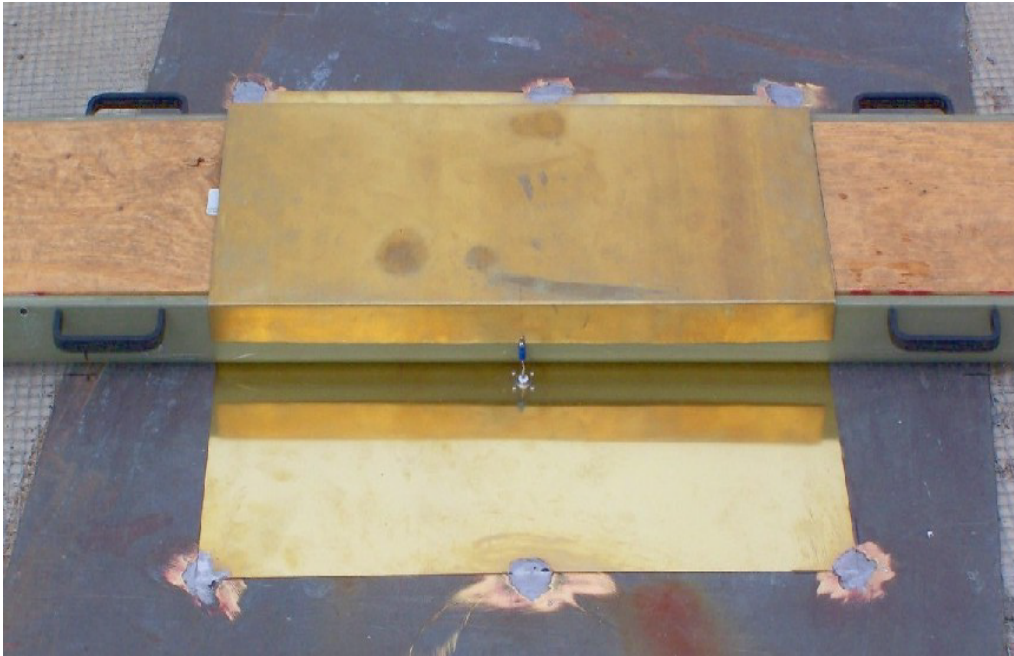
Figure 2: Closeup of the feed point in the Surface Probe.
