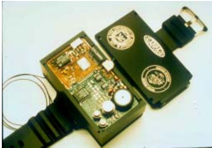
Figure C.22. A wearable wireless microinstrumentation system (Mason et al. 1998).
