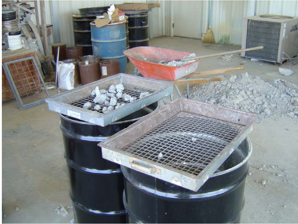
Photo 2. Processing the RCP to determine gradation
