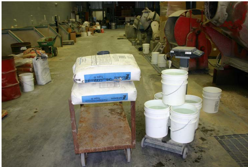
Photo 10. Obtaining the correct amount of water for proportioning the Type III portland cement grout
