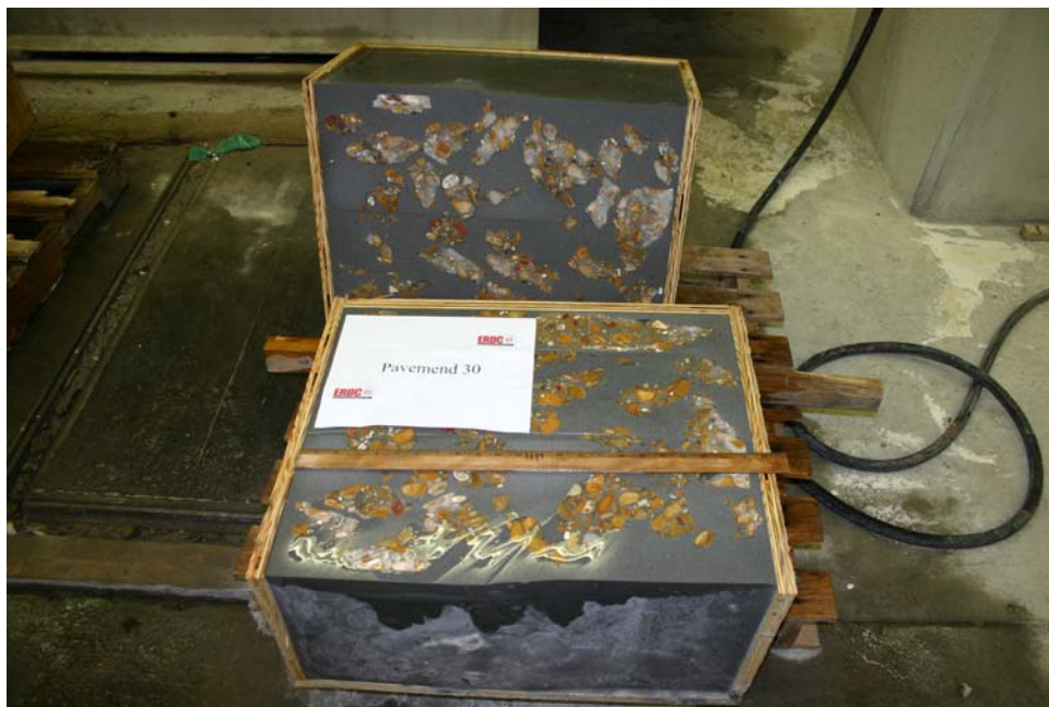
Photo 13. Box 1 cut in half to permit inspection of impregnation
