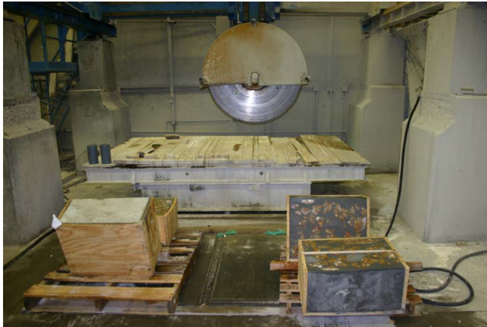
Photo 12. Large diameter concrete saw used to slice the box samples for inspection
