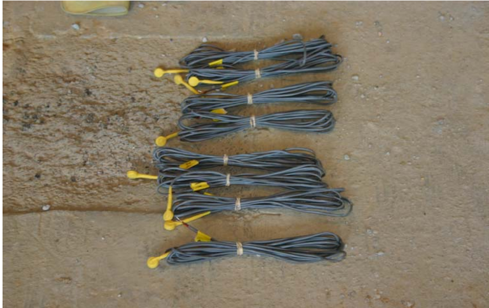
Photo 32. Sensors used to measure and record temperature in the repairs
