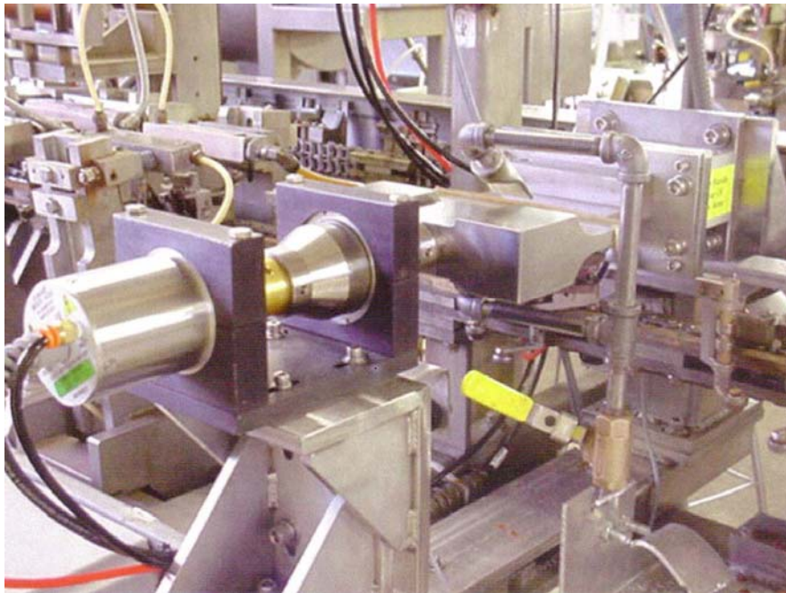
Figure 13. Ultrasonic Sealing Module Integrated in MRE Packaging Line
