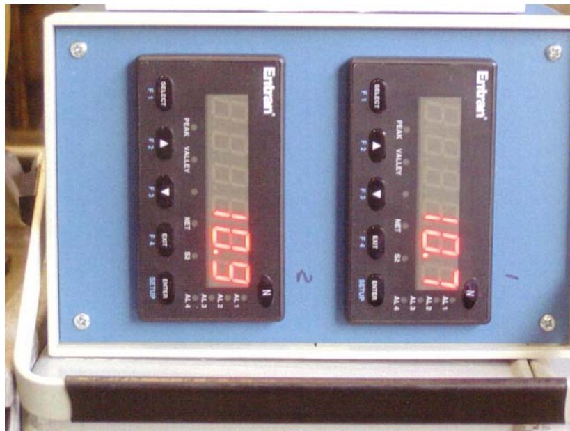
Figure 21. Left and Right Ends Force Readings are Close to Each Other (The two values indicate the amount of pressure each load cell experiences during the pressure application of the seal.)
