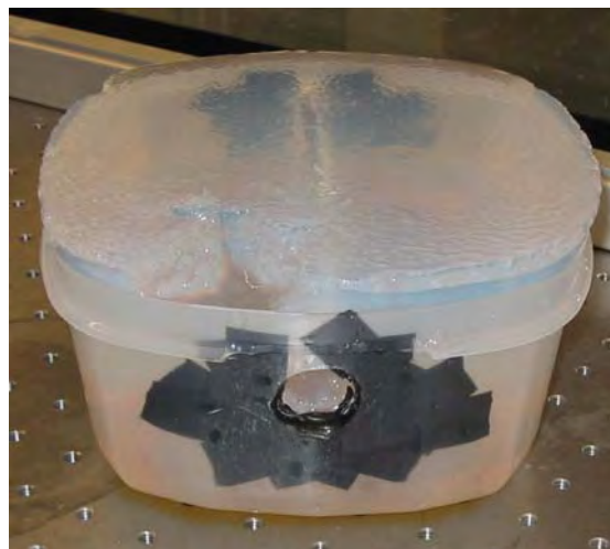
Figure 19: Prostate phantom- a photographic view.
