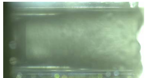
Figure 7: A sample photograph from the experiments showing the chaotic surface associated with operating conditions with good atomization. Flow moves from left to right.
