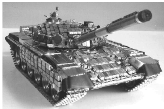
Fig. 6. Photo of one of the scaled T-72 BK's used to test the full ATR algorithm.
