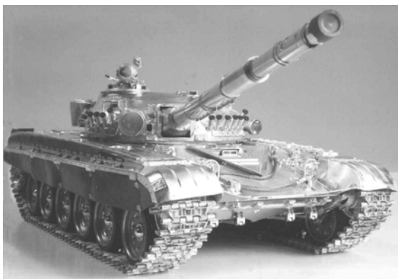
Fig. 5. Photo of one of the scaled T-72 M1's used to test the full ATR algorithm.
