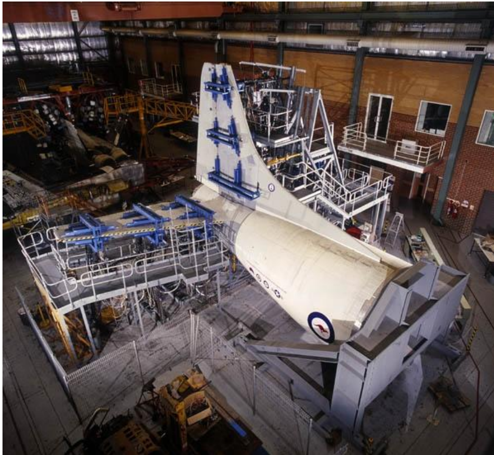
Figure 21: P-3C Empennage fatigue test at DSTO
