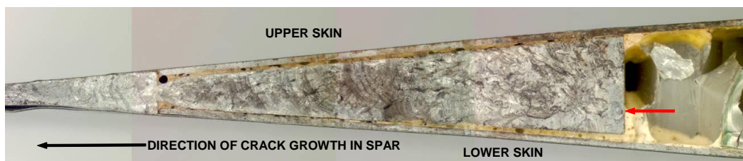
Figure 35: Composite photograph showing an overall view of the fracture surface of the crack in the trailing edge spar. Note the presence of progression marks clearly indicating that cracking was due to fatigue. The origin of the crack is indicated by the red arrow
