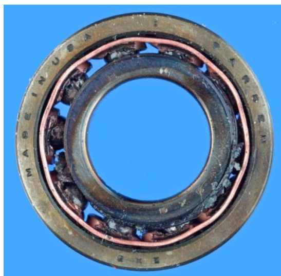
Figure 45: Photograph of a bearing from the Turbo Compressor which had been severely damaged by overheating
