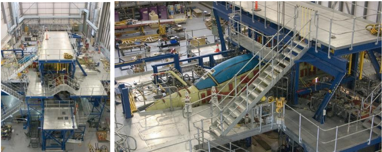
Figure 33: LIF Test Rig (left) under construction, and (right) with aircraft installed.
