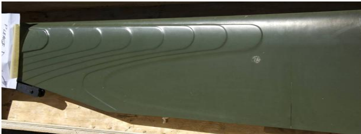
Figure 34: Photograph of the crack (lower right, vertical on page) in the MRB showing its location in relation to the blade root
