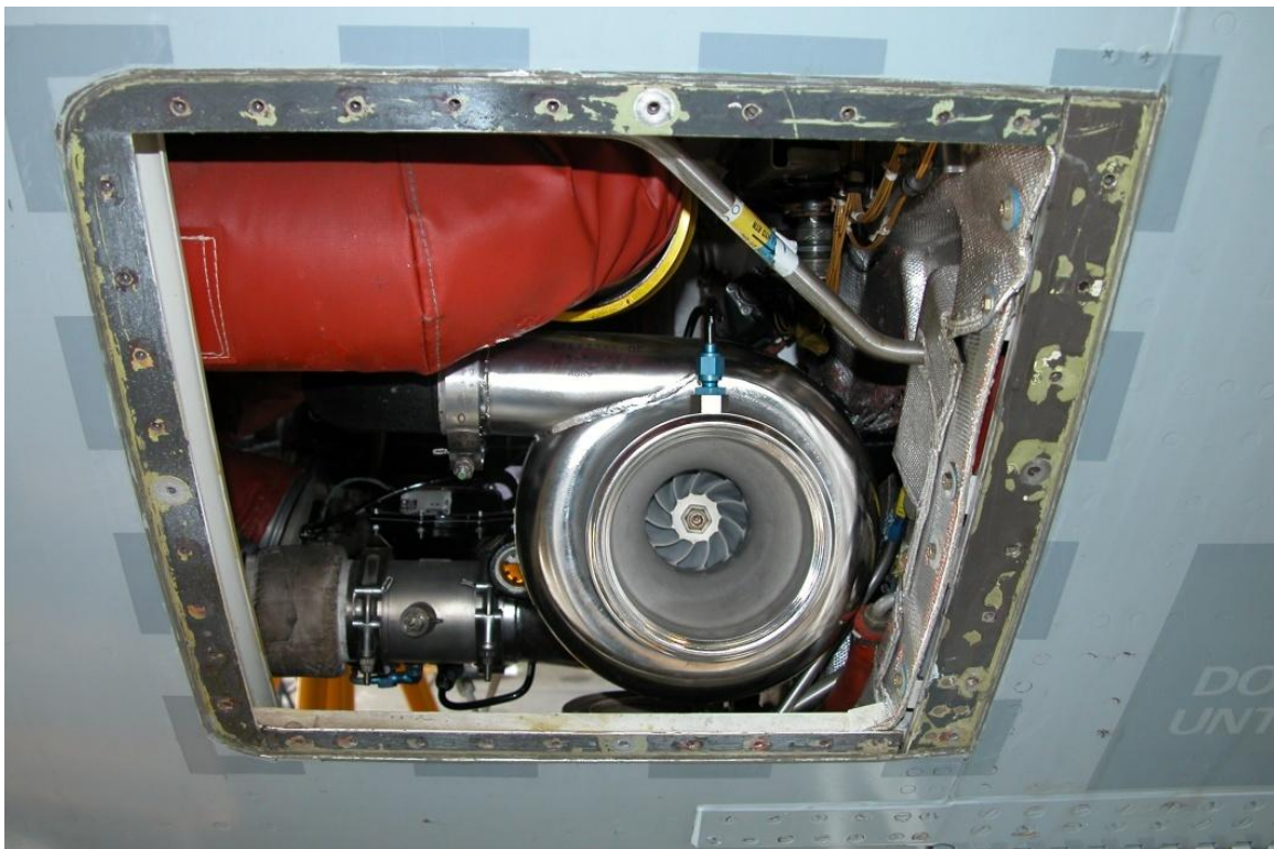
Figure 42: Photograph showing the compressor inlet (arrowed) in situ on the port side of an aircraft
