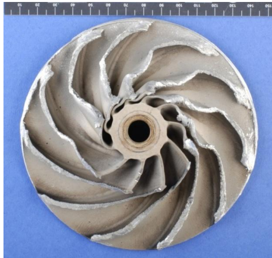
Figure 43: Photograph showing impeller vane damage from Turbo Compressor
