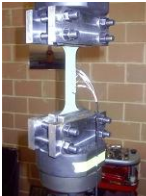
Figure 63: POD test coupons during fatigue testing
