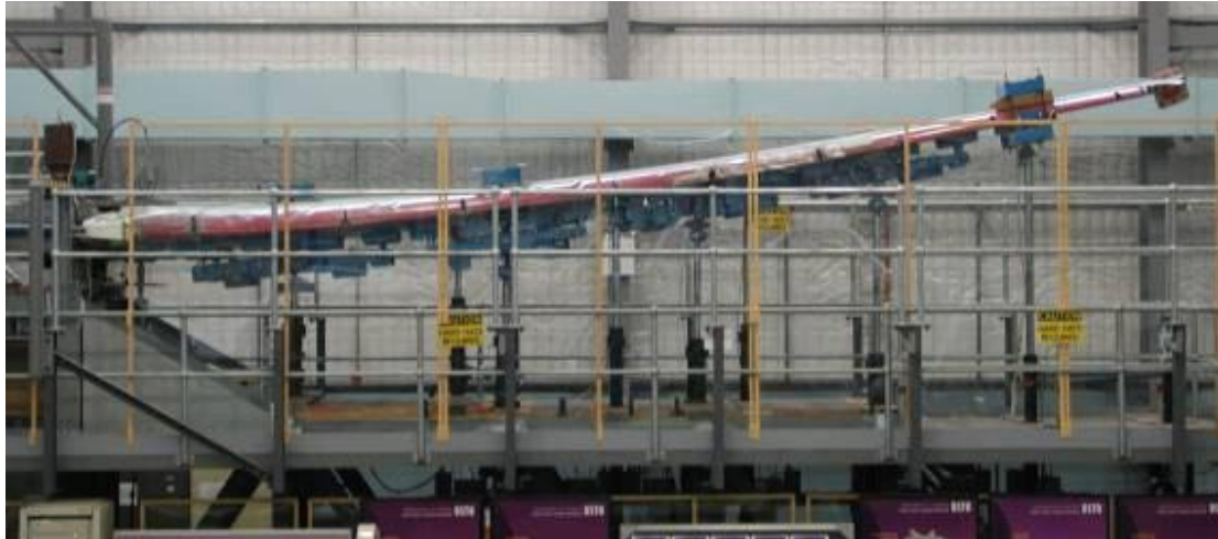
Figure 5: F-WELD Test Article Undergoing Cold Proof Load Test
