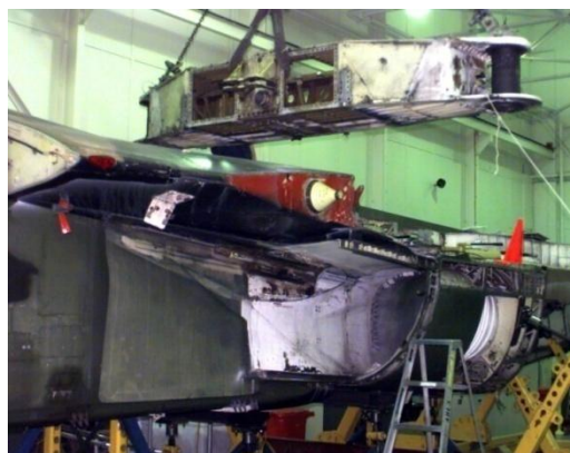
Figure 12: Arrival of the teardown aircraft, and removal of wing carry-through box
