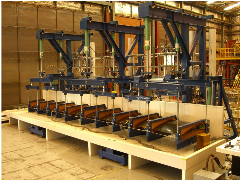
Figure 53: The Pre-production Outboard Flap Test Rig
