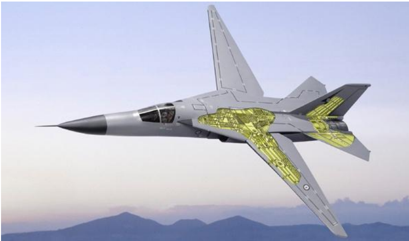
Figure 11: F111C in RAAF configuration showing critical structural areas
