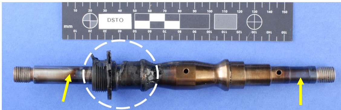
Figure 44: Photograph of severely heat damaged shaft from the Turbo Compressor
