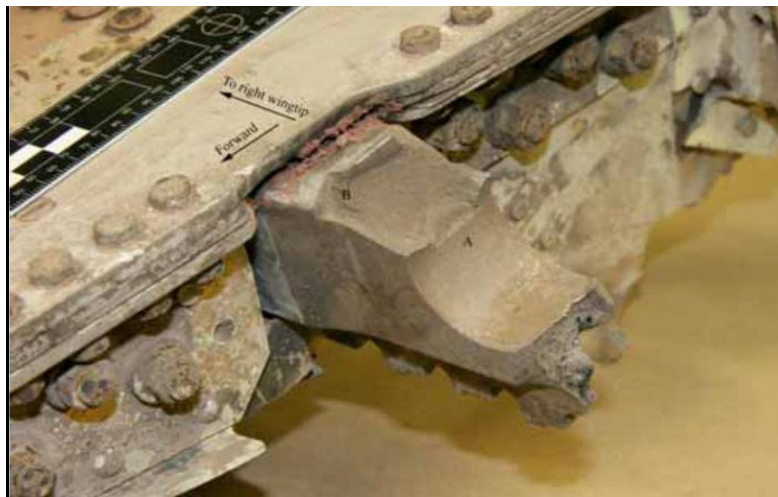
Figure 55: Broken lug on the inboard end of the right wing
