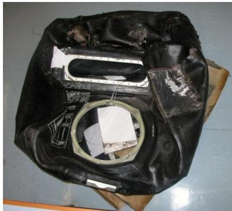
Figure 40: Photograph of the Black Hawk Port Fuel Cell in the collapsed condition with no external cover or packaging. The cell contained a small amount of water and dirt
