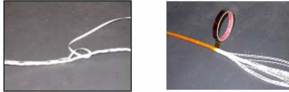
Figure 4 Cable construction: (a) lacing; (b) Kapton wrap
