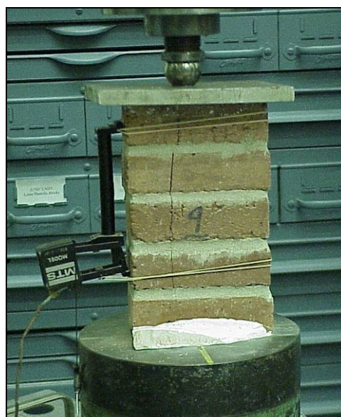
Figure 2-15. Compression test of prism.
