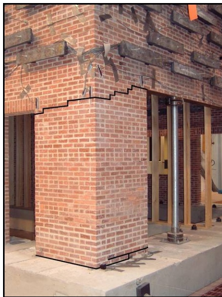
Figure 6–19. Crack pattern on pier 12 and pier 4 indicating structural continuity.
