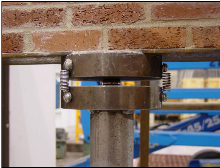
Figure 2-7. Pin connection for steel support column.
