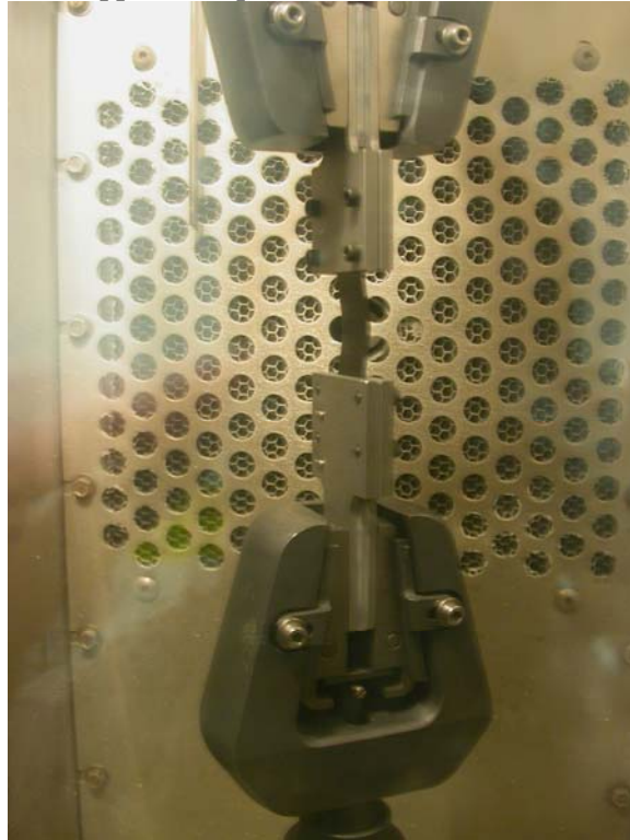
Figure 4: Buckling test setup showing buckled sample.
