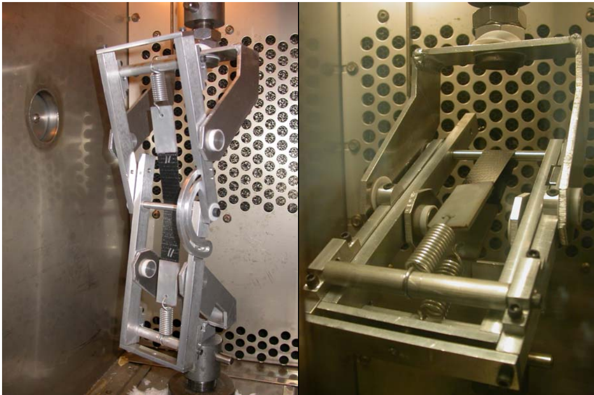
Figure 8: Folding apparatus within the environmental chamber and shown first unfold and second, folded.
