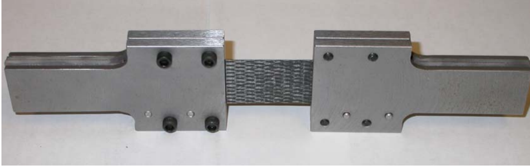
Figure 3: Buckling test fixed-fixed support clamps.
