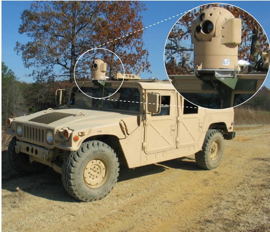
HTSS gimbaled sensor platform mounted to test vehicle
