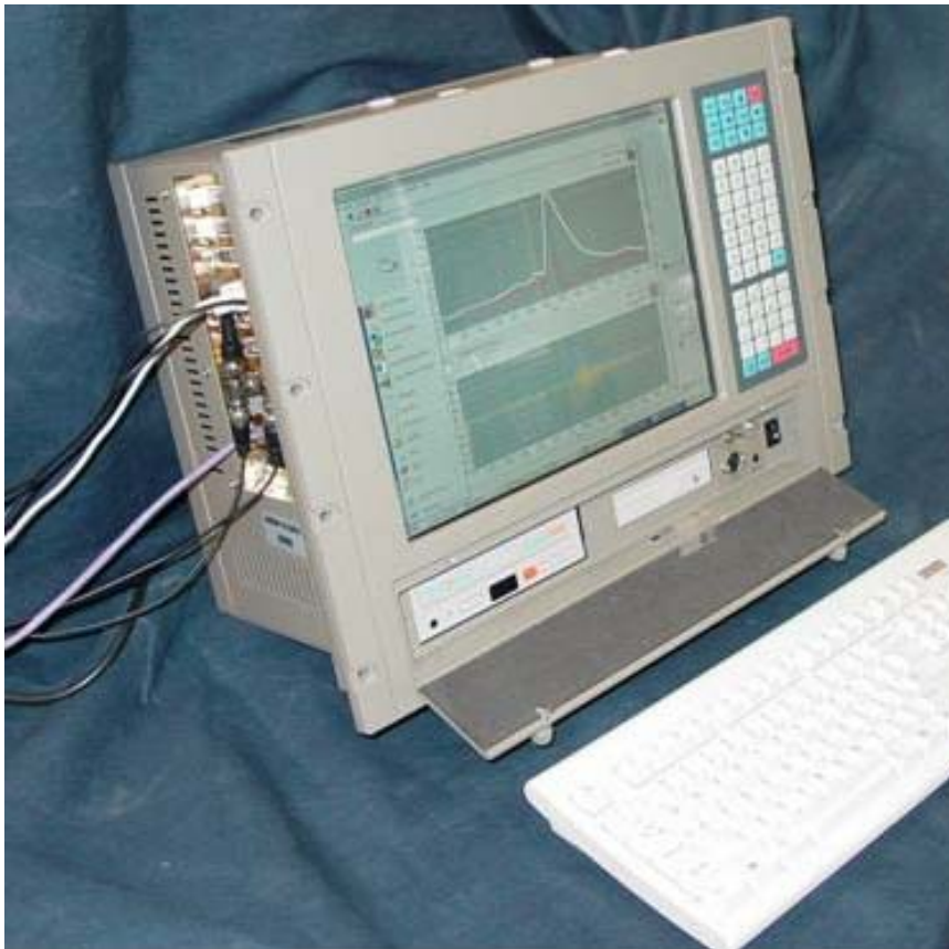
Figure 5. Portable acoustic test system.
