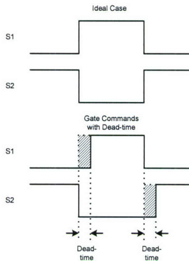
Fig. 6-8. Application of dead-time in gate waveforms.
