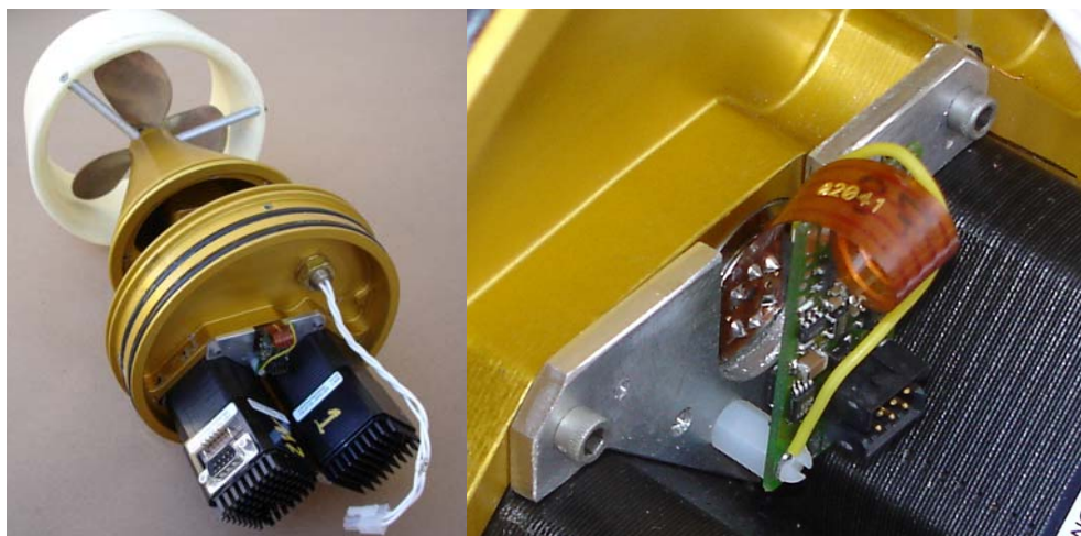
Figure 2.2.8: Pressure Sensor Integrated in RPUUV Tail Section
