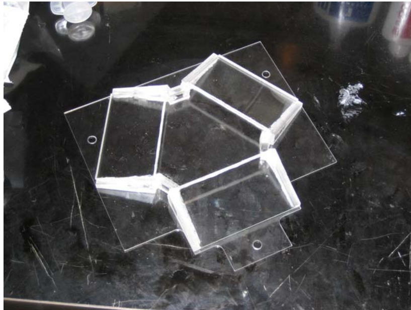
Figure 37. Water-filled prism design for 3DDLCPTV camera
