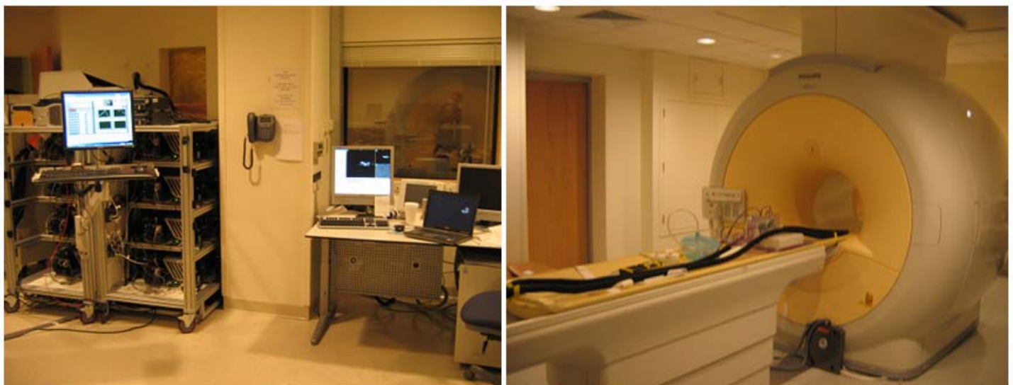
Fig. 3. Photographs of the spectroscopy system (left) in the MR control room. The fibers run through Ports in the wall into the MR bore (right).
